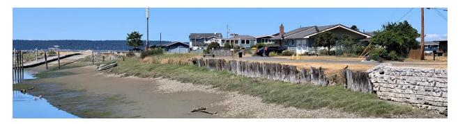
Seashore Ave and the canal shoreline are not in imminent danger of catastrophic erosion. Some minor improvements such as repairing the end of the block wall, pulling some invasive weeds and repairs to portions of the boat launch dock decking can occur ahead of the rest of the repairs.
